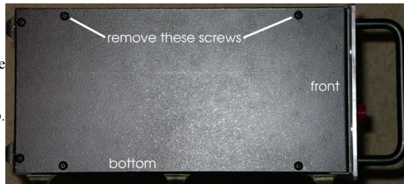
Figure 10 - Remove these side screws on both sides
