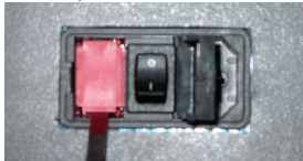
Figure 3 - Pop fuse block up with screwdriver
