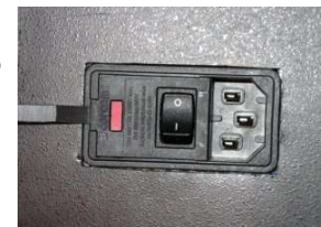
Figure 2 - Swing open fuseholder door with screwdriver
