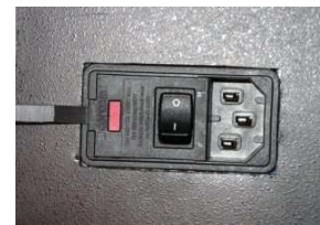
Figure 6 - Swing open fuseholder door with screwdriver
