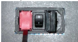
Figure 7 - Pop fuse block up with screwdriver
