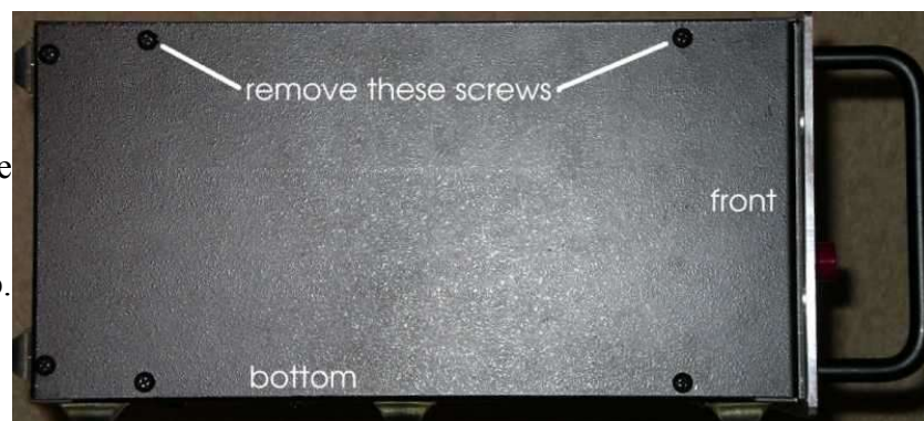
Figure 10 - Remove these side screws on both sides
